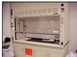
For optimal fume hood operation, keep laboratory doors closed at all times.
